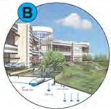
B Roof Runoff Water will be collected from the roof and piped to an underground cistern that is connected to an irrigation system. Once the cistern is full, excess roof water will be diverted to the bioswale.
