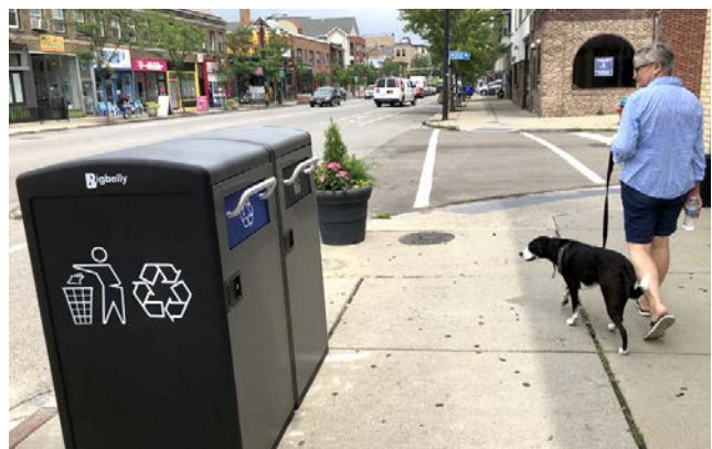
Example of SC-SC Double Station with SC Hopper for Recycling and SC Hopper for Trash
